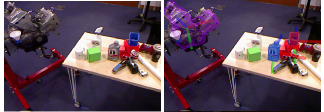
Fig. 1: Given an RGB image (left) and depth frame, our SegICP approach segments the objects in a pixel-wise fashion and estimates the 6 DOF pose of each object with 1 cm position and 5^\circ angle error (right).
