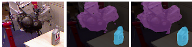
Fig. 6: SegNet and DilatedNet: outputs respectively (middle, right) given the same input RGB input image (left) from the PR2’s Kinect1; SegNet appears to generate tighter segmentation compared to DilatedNet.
